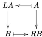
The lines with ‘%D 2Dx’ and ‘%D 2D’ define a grid with coordinates and nodes, and the lines between ‘%D ((’ and ‘%D ))’ connect these nodes with arrows.
